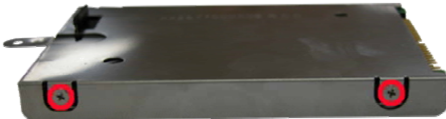
Fig. 5 Unscrewing the hard disk drive bracket screws
